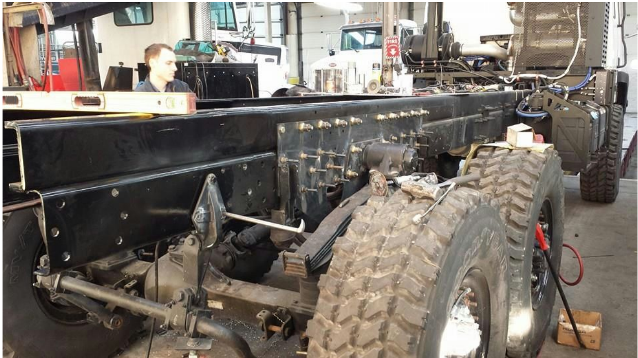
Starting the reassembly phase. The rear axle and suspension assembly is being installed in its new position. Our tech is using OEM style Huck fasteners for factory look and strength.
