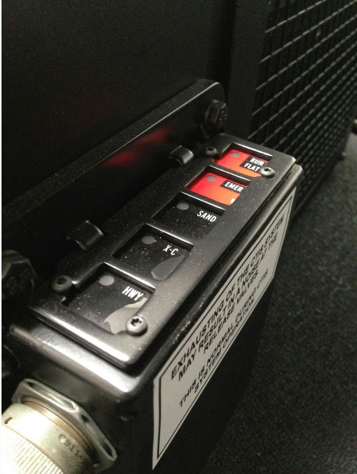
Shot of CTIS system. This BAE 6x6 is manufactured with CTIS installed as part of the base model of the truck.
