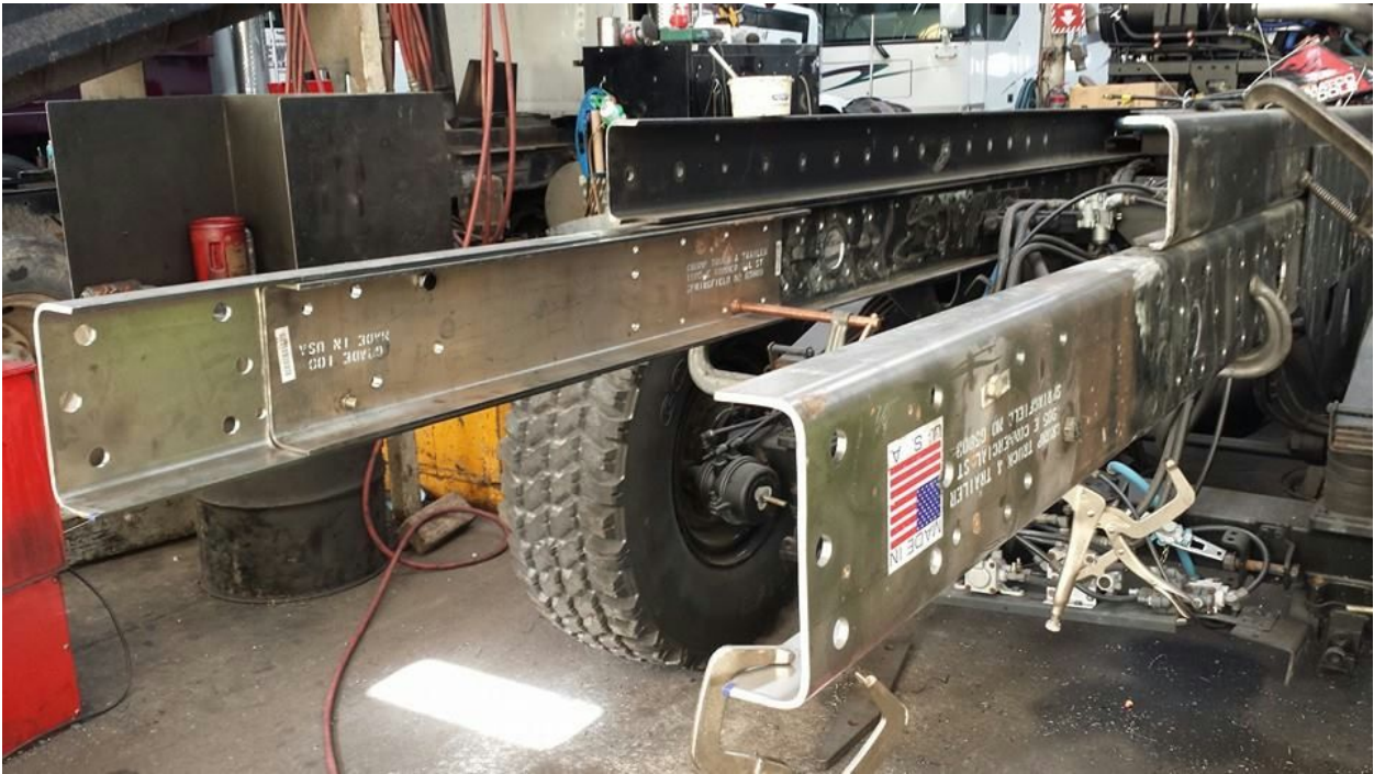
Laying out the reinforcements for the lower rails and drilling holes!
