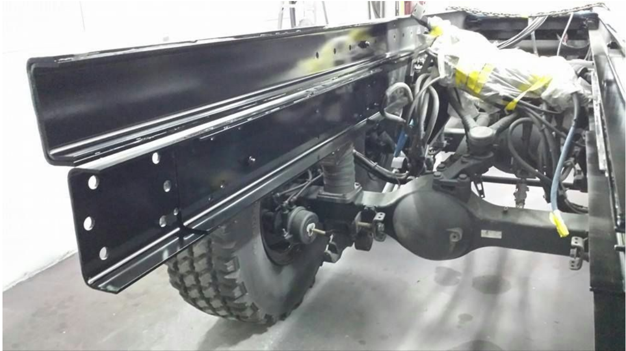
Starting the reassembly phase. The rear axle and suspension assembly is being installed in its new position. Our tech is using OEM style Huck fasteners for factory look and strength.
