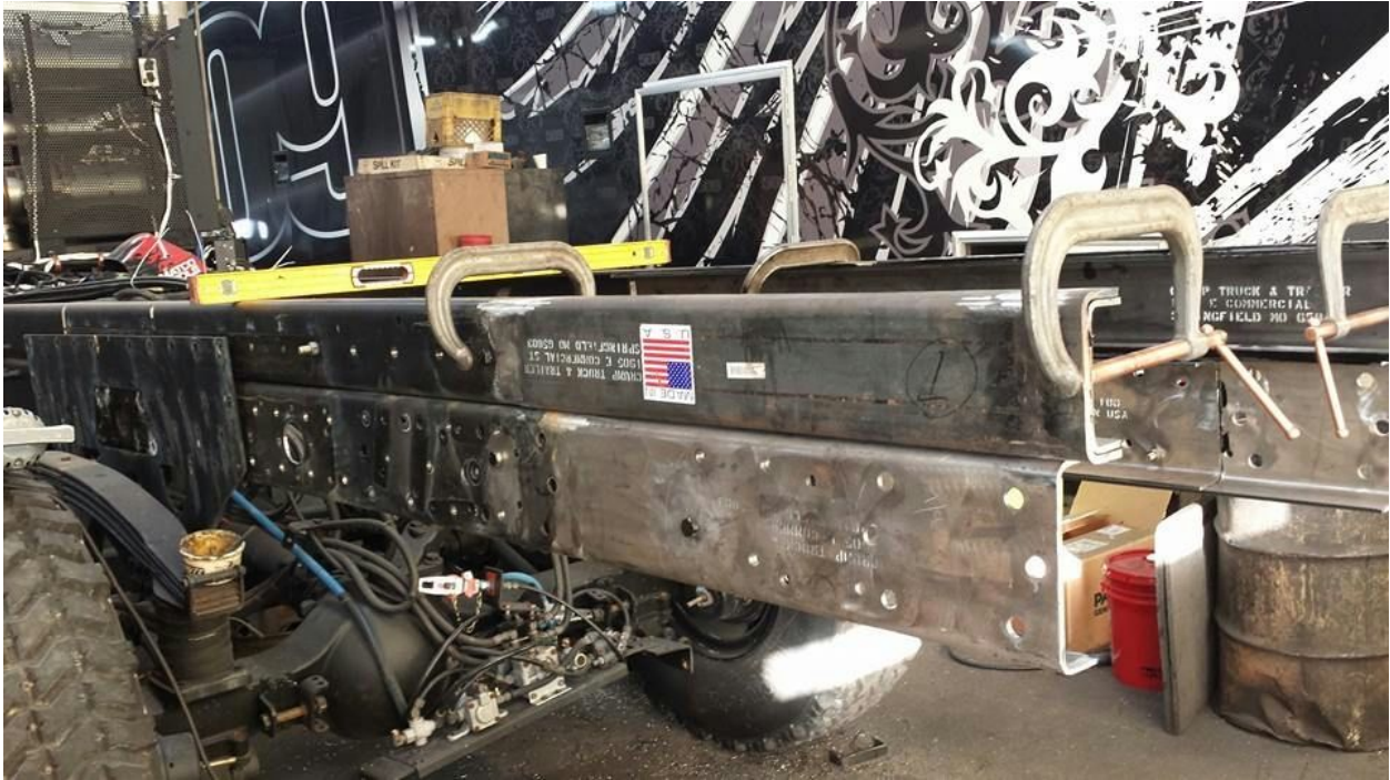
Adding on the upper rail extensions.
